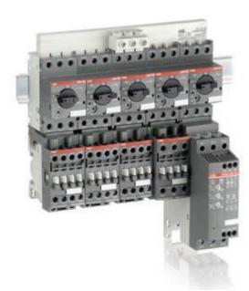
These devices are mainly used to switch motors manually on/ off and protect them against short-circuit, overload and phase failures. Fuse less protection with a manual motor starter saves costs, space and ensures a quick reaction under short-circuit condition, by switching off the motor within milliseconds.
